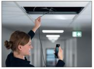
Cable Scout Cam is a professional WiFi HD inspection camera for visual inspection of objects up to 10 meters away. It is possible to transmit video images in real time and take video and photo shots in confined spaces that would otherwise be difficult to view. This product is compatible with Android, iOS, Windows and MAC operating systems.
